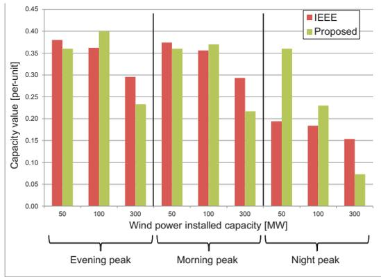
Fig. 3. Capacity Value [pu] of “El Arrayán” wind farm using the proposed and the IEEE method
