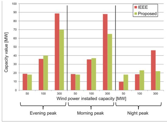
Fig. 2. Capacity Value [MW] of “El Arrayán” wind farm using the proposed and the IEEE method
