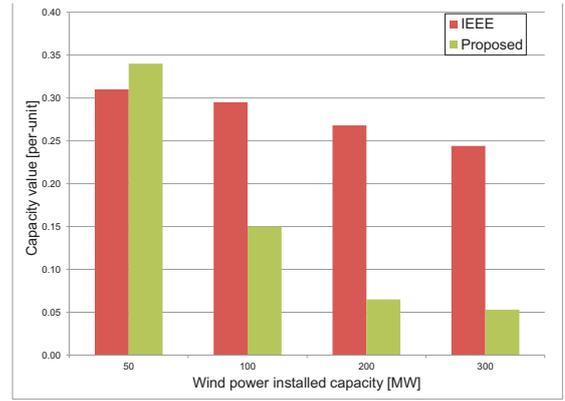
Fig. 4. Capacity Value of “Lebu Sur” wind farm using the proposed and the IEEE method
