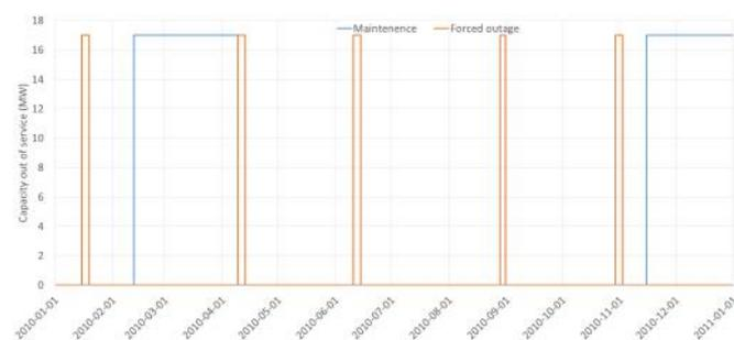
Fig. 5. Maintenance and forced outages for Kakira bagasse steam generator
