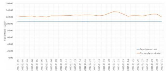
Fig. 6. Fuel offtake (GTP + industrial demand) with and without gas supply capacity constraint at Songo-Songo
