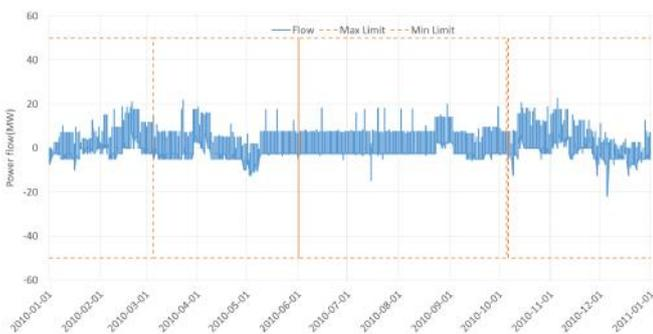
Fig. 4. Rwanda-Eastern DRC power flow (2010 existing interconnectors scenario)
