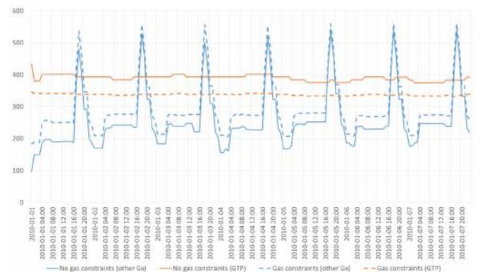
Fig. 7. Representative week of Tanzania generator dispatch (with and without gas supply capacity constraints)
