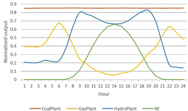
Figure 12. Normalised average hourly load profile for 20% penetration scenario with solar only and a full energy mix (coal, gas, hydro)
