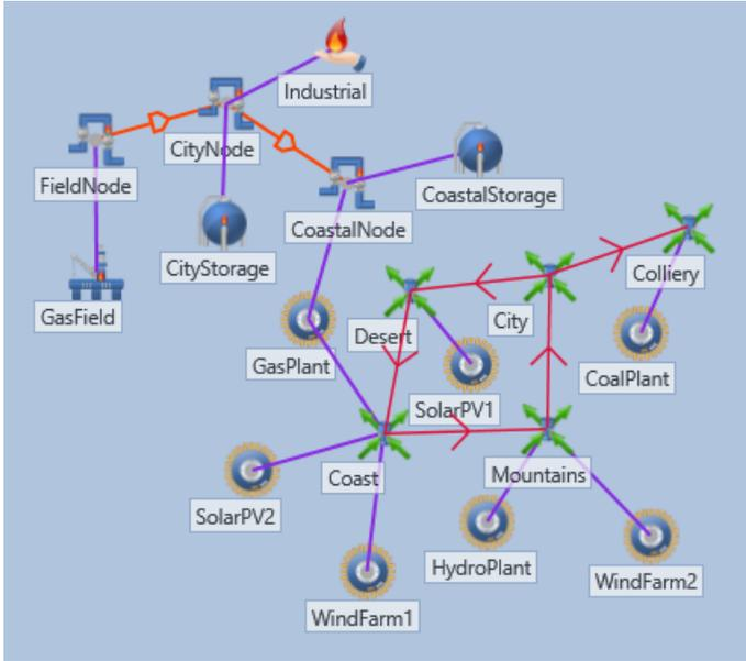
Figure 2. Overview of the gas-electric representative model in PLEXOS® Integrated Energy Model
