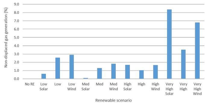
Figure 6. Non-displaced gas-fired generation for different RE penetration scenarios
