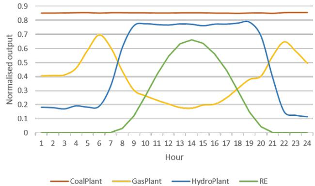
Figure 11. Normalised average hourly load profile for 10% penetration scenario with solar only and a full energy mix (coal, gas, hydro)
