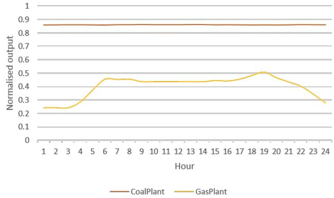
Figure 10. Normalised average hourly load profile for no RE penetration scenario with a limited energy mix (coal, gas)
