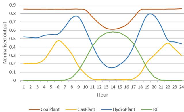
Figure 14. Normalised average hourly load profile for 40% penetration scenario with solar only and a full energy mix (coal, gas, hydro)
