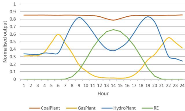
Figure 13. Normalised average hourly load profile for 30% penetration scenario with solar only and a full energy mix (coal, gas, hydro)
