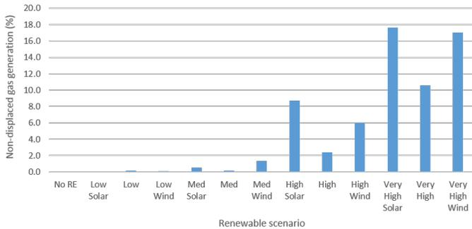
Figure 8. Non-displaced gas-fired generation for different RE penetration scenarios
