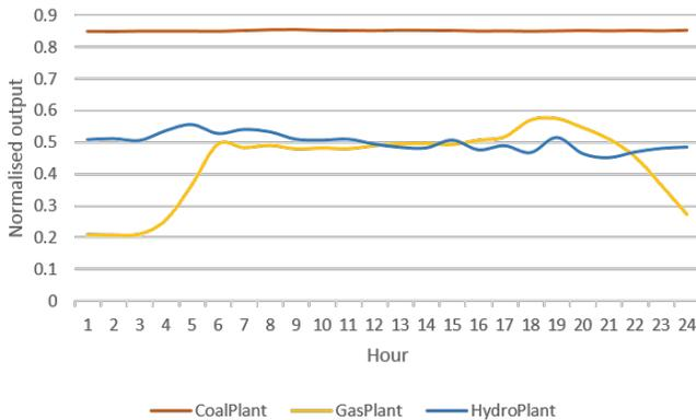
Figure 9. Normalised average hourly load profile for no RE penetration scenario with a full energy mix (coal, gas, hydro)
