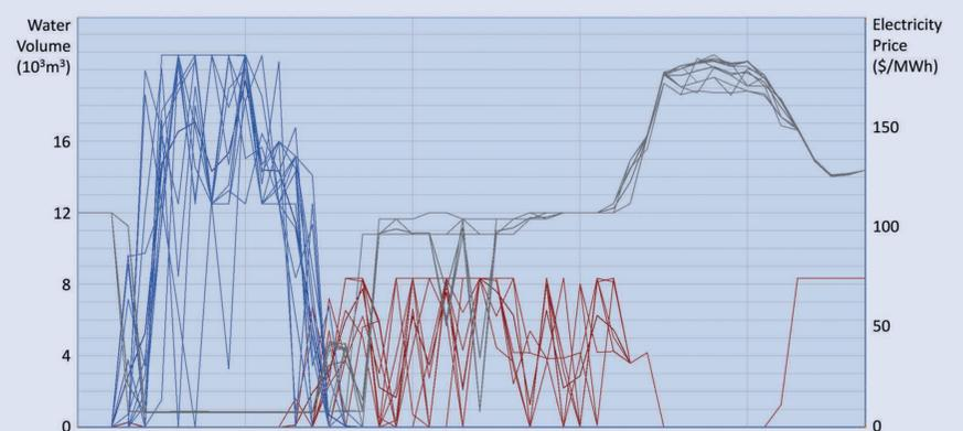
**Figure 02 – Stochastic Optimisation's water injection (blue) and withdrawal (red) over electricity prices (grey).**
