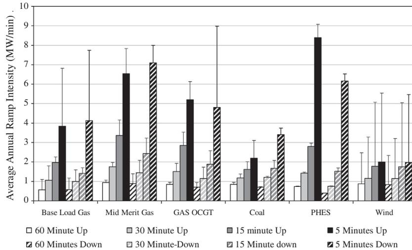
Fig. 3. Modelled annual average ramping intensity (up and down) for each simulation configuration for each generation type.
