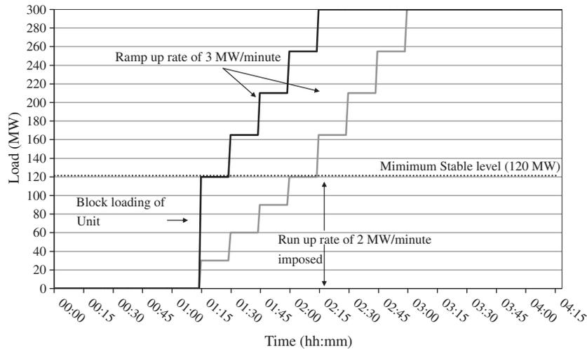
Fig. 1. Example of run up rate and block loading for a thermal unit.
