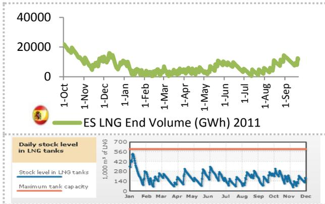
Figure 4: LNG Storage pattern (Upper Plexos Model 2011-2012, Bottom Enagas 2012 [4]s)
